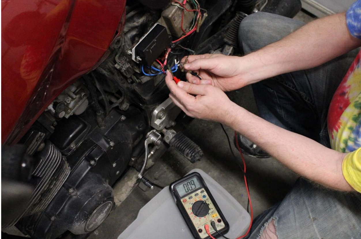
Figure 4 - Measuring the stator winding resistance
