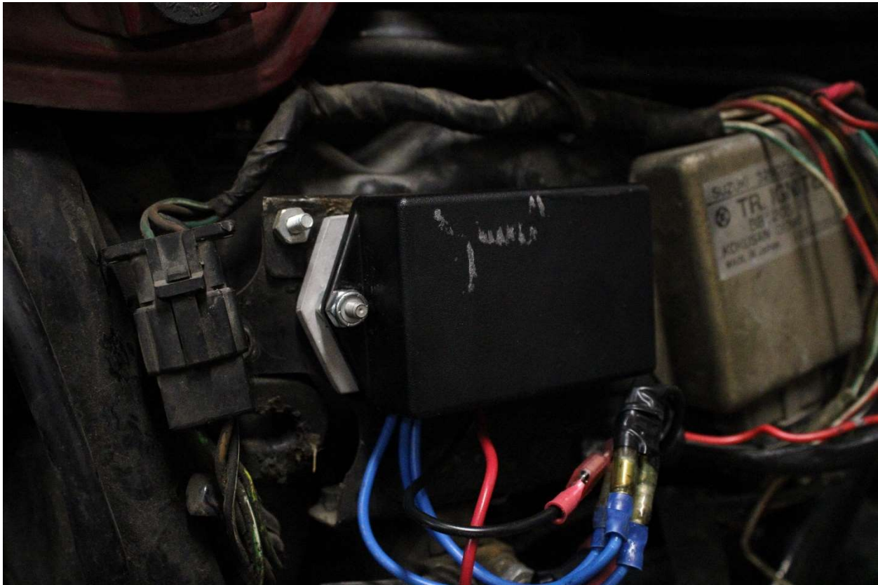
Figure 8 - Attach regulator to mounting plate and connect wires
