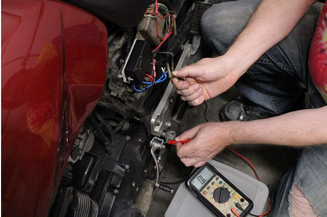
Figure 3 - Measuring resistance from stator winding to ground
